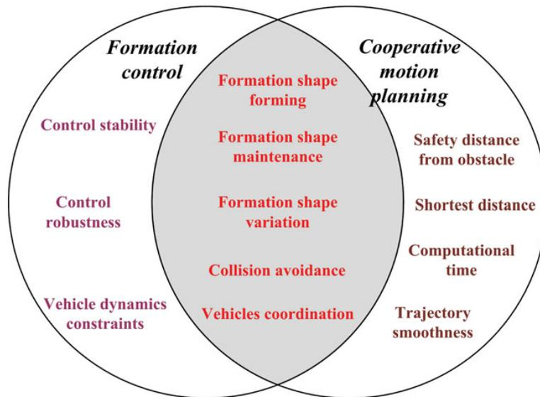
Figure 5: Overlap between formation control and cooperative motion planning, Liu et al.[2]
