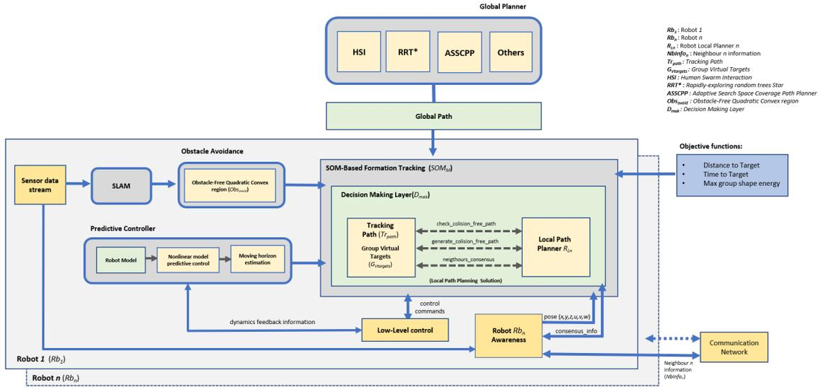
Figure 6: Purposed SOM-based formation tracking system architecture overview.
