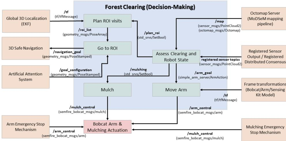
Figure 9: Ranger’s Decision-Making Process for Forestry Clearing.
