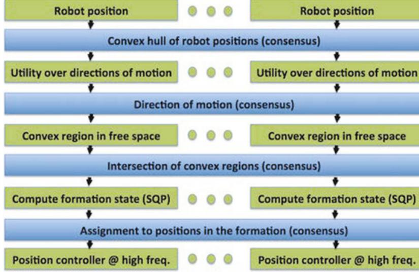
Figure 16: Schema of the convex obstacle free method.
