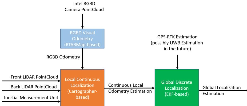
Figure 1: Proposed local and global fusion approach for 6D full pose localization estimation in SEMFIRE.
