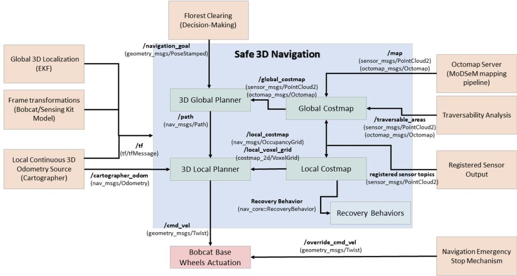
Figure 8: Ranger's Safe 3D Navigation Architecture.
