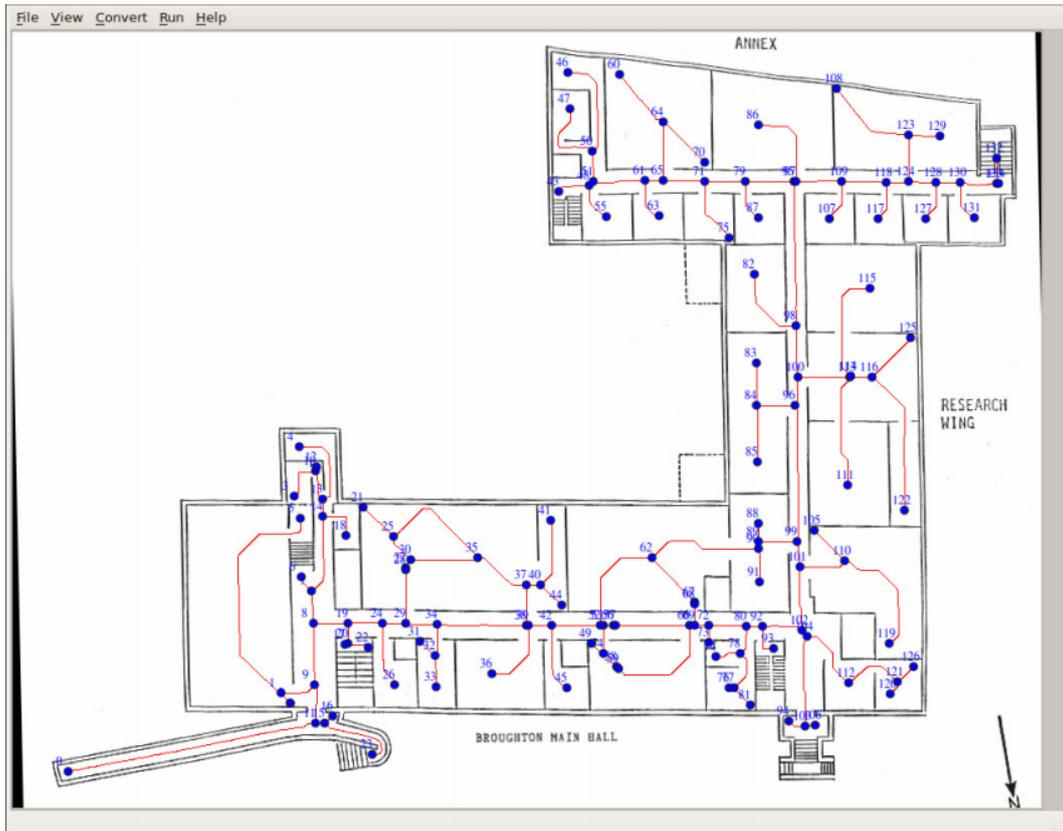
Figure 7: A patrol graph displayed on top of a metric map to be used in multi-robot patrolling tasks. The blue dots represent the vertices of the graph that must be visited, while the red arcs represent the edges that connect pairs of vertices [254].
