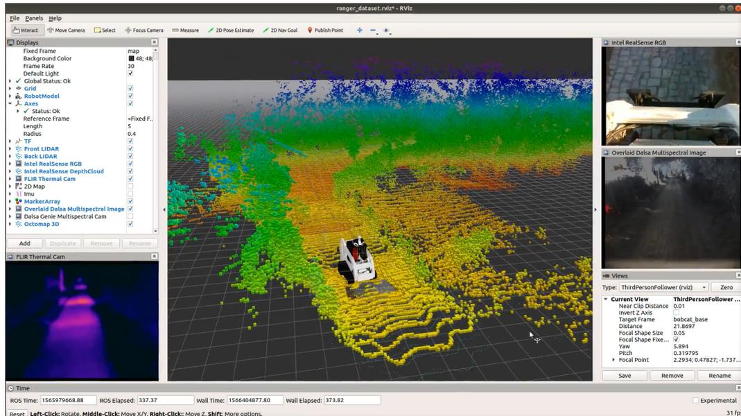
Figure 3: Results of initial tests with a 3D map of a challenging outdoor environment using the proposed localization and mapping approaches.
