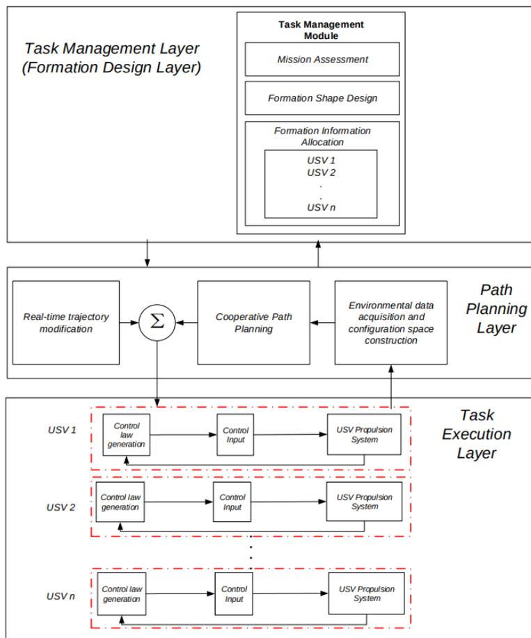
Figure 12: Multi-robot formation example architecture, from Liu et al. work.
