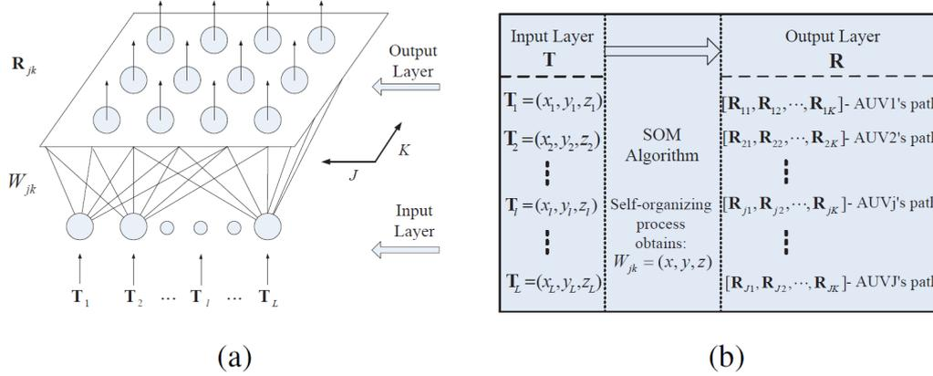
Figure 14: SOM neural network (a) structure and the (b) mapping relationship of the two layers, presented in [3] work.
